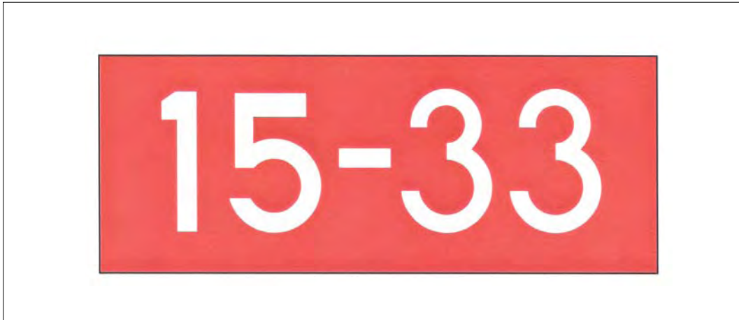
FIG 2-3-24 Runway Holding Position Sign
