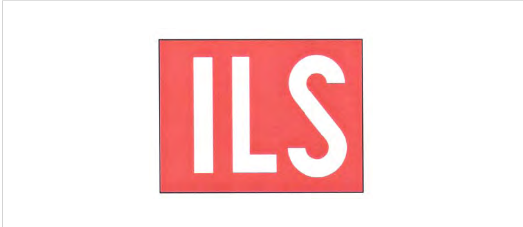
FIG 2-3-28 Holding Position Sign for ILS Critical Area
