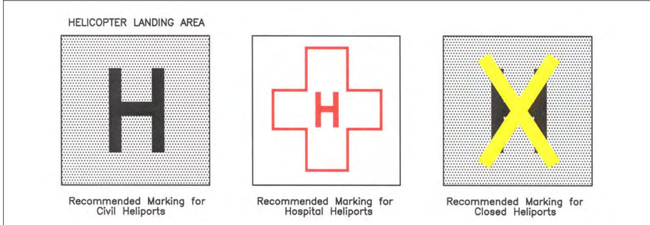
FIG 2-3-23 Helicopter Landing Areas
